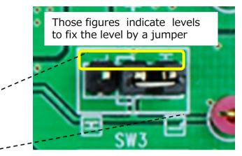
On this evaluation board, jumpers as shown in the picture above are provided for setting operation of TB67S261FTG
