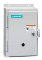
Non-reversing NEMA contactor, Size 1, Three phase full voltage, Contactor amp rating 27A, 3 wire (NO aux included), 110-120/220-240VAC 60Hz coil, Non-combination type, Enclosure NEMA type 12, Dust/drip proof for indoors, Extra-wide enclosure
