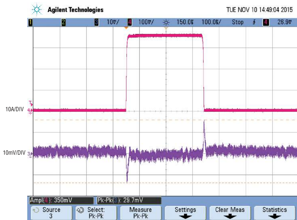
Figure 5. Load Transient Waveform of DC2291A, V_{IN} = 12V , V_O = 1.0V , F_{SW} = 450kHz , 0% to 25% (0A to 35A) Load Step
