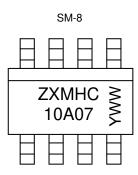
$\begin{array}{l} \text{ZXMHC10A07} = \text{Product Type Marking Code} \\ \text{YWW} = \text{Date Code Marking} \\ \text{Y or } \overline{\text{Y}} = \text{Last Digit of Year (ex: 5= 2015)} \\ \text{WW or } \overline{\text{WW}} = \text{Week Code (01~53)} \end{array}$
