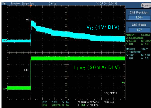
FIGURE 22. LOAD REGULATION WITH I_{LED} CHANGES FROM 0% TO 100% PWM DIMMING
