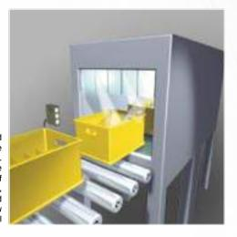
Machines in the food industry need to be cleaned frequently. With rapid temperature changes, and lots of water and steam, a completely sealed sensor with window heating is essential
