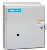
Mechanically held lighting contactor, Contactor amp rating 30Amp 0NC \_ 2NO poles, 440VAC 50HZ/480VAC 60HZ coil, Non-combination type, Enclosure NEMA type 12, Dust/drip proof for indoors
