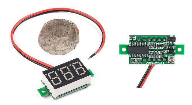
**Description:** This Digital LED Voltmeter measures the voltage at a particular point of the system it has been hooked up to and then provides a readout on its three 7-segment LEDs. This voltmeter is able to provide a readout of voltages from 2.5VDC to 30VDC within a 1% accuracy.
