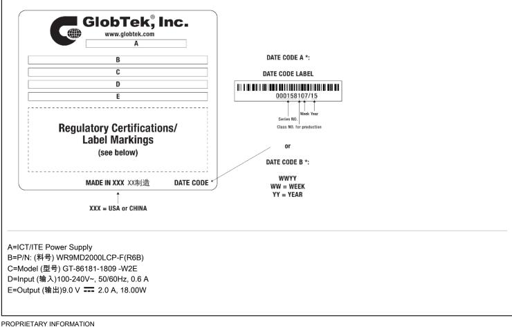
PROPRIETARY OF GLOBTEK, INC. ANY REPRODUCTION, DISCLOSURE OR USE OF THIS DRAWING, IN WHOLE OR IN PART, IS HEREBY PROHIBITED EXCEPT AS SPECIFIED IN Page 11 of 15 WRITING BY GLOBTEK, INC. © GlobTek, Inc. 2019 - 2023
