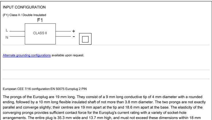
behind its front plane (this allows for the recesses on many European socket types). The left and right side of the plug are formed by surfaces that are at 45° relative to the horizontal plan.
