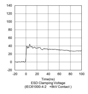
ESD Clamping Voltage VCL(V)
