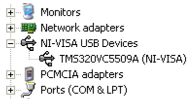
Figure 10. NI-VISA Driver Verification Using Device Manager
