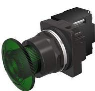
30mm BlackMax, Epoxy Coated Corrosion Resistant Metal Operator, Round Illuminated Twist-to-Release Full Voltage, 6V AC LED Lamp Mushroom Head Cap Small 1.79" (45 mm) Plastic Cap, Green 2 Position Maintained, Twist-to-Release UL Listed, CSA Certified NEMA 1,3,3R,4,4X,12,13 & Automotive Standards
