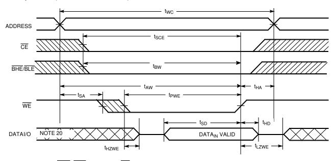
Write Cycle No. 4 ( $\overline{BHE}$ -/ $\overline{BLE}$ -controlled,  $\overline{OE}$  LOW)[17, 18]
