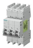
Miniature circuit breaker 240 V 10kA, 3-pole, D, 32 A, D=70 mm according to UL 489  $\,$
