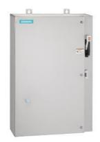
Non-reversing motor starter Size 1 Three phase full voltage Solid-state overload relay OLRelay amp range 5.5-22A Combination type 30Amp non-fusible disconnect Encl NEMA type 4X 316 S-steel Water/dust tight non-corrosive Extra-wide enclosure
