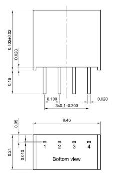
Projection: Third angle projection Unit: inch PIN tolerance:  $\pm 0.004$ Tolerance: X.XX  $\pm 0.02$  X.XXX  $\pm 0.01$
