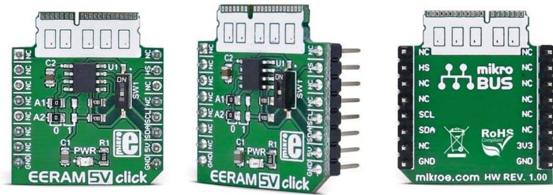
Add memory to your project with **EERAM 5V click**. It carries the 47C16 EERAM, a 16Kbit SRAM with EEPROM Backup from Microchip. The click is designed to run on a 5V power supply. It communicates with the target microcontroller over I2C interface, with additional functionality provided by the INT pin on the mikroBUS™ line.
