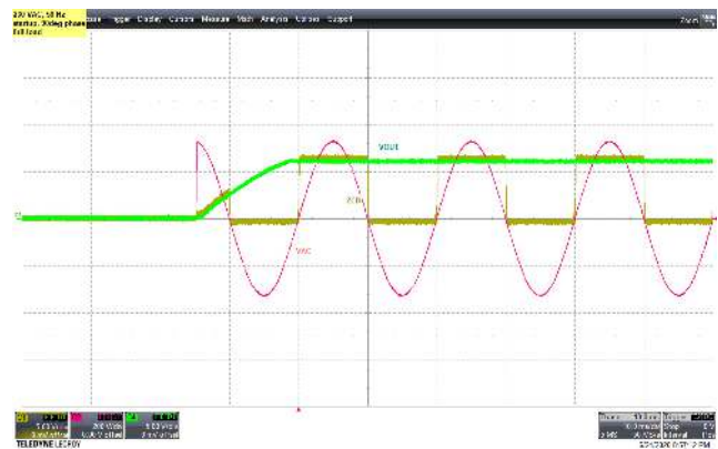
Figure 21 – 230 VAC 50 Hz, Full Load. CH1: ZCD, 5 V / div., 5 ms / div. CH2: V_{IN} , 100 V / div., 5 ms / div. CH4: V_{OUT} , 5 V / div., 5 ms / div.
