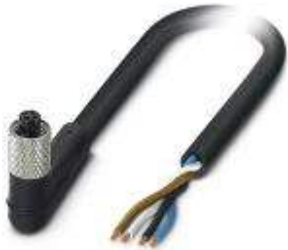
Sensor/Actuator cable, 4-position, PUR, Black RAL 9005, Free cable end, on Socket angled M5, A-coded, Cable length: 1.5 m
