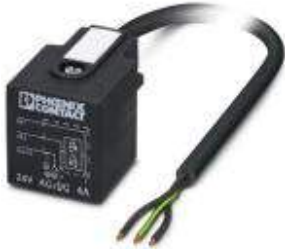
Sensor/Actuator cable, 3-position, PVC, Black RAL 9005, Free cable end, on A valve plug, with 1 LED, connected with Z diode, Cable length: 2 m
