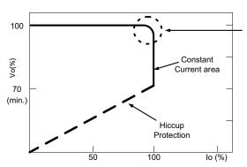
Typical LED power supply I-V curve
