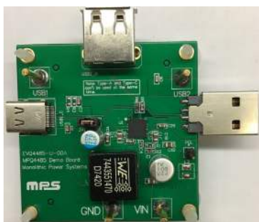
(L x W x H) 5cm x 5cm x 1.7cm (Four Layer PCB/2oz per layer)
