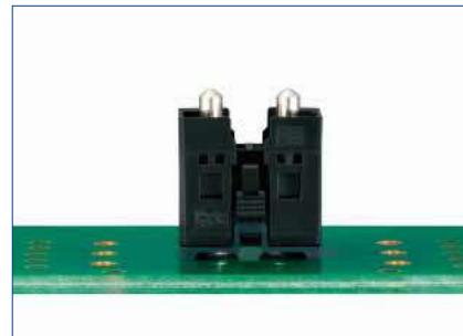
③ Interposer Installed
