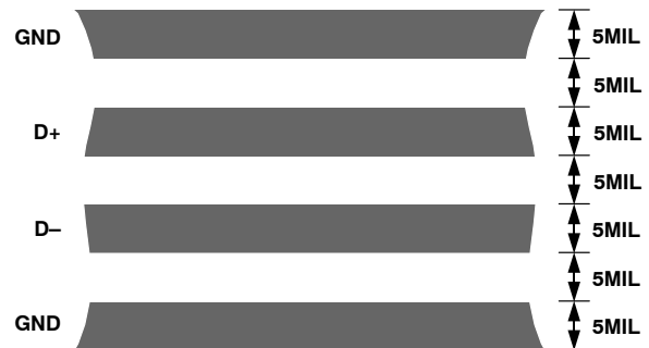
Figure 21. Typical Arrangement of Signal Tracks
