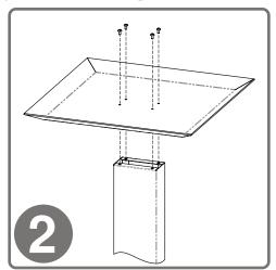
Use Phillips screwdriver to secure base to column with (4x) screws  $(10-32 \times 5/16")$ .
