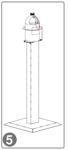
Bottles can be secured with a zip-tie or cable from the handle to the top ring, if added security is needed.
