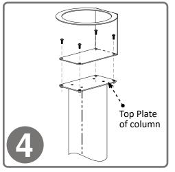
Attach the BW004-0512 Bottle Holder to the column using (4x) screws included with stand. Tighten.
