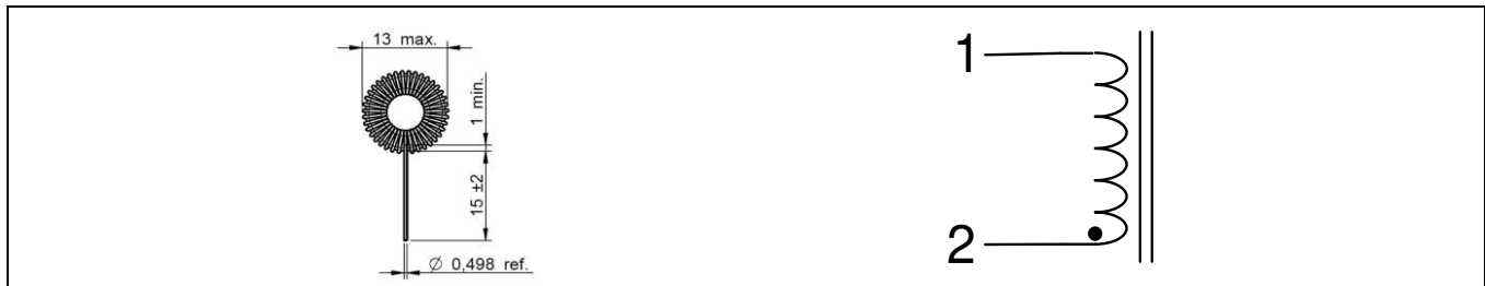
Figure 13 DM choke (side view) and electrical diagram
