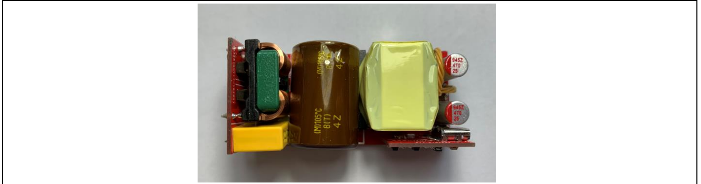
Figure 1 REF_XDPS21081_65W FQR ZVS flyback converter (top view)
