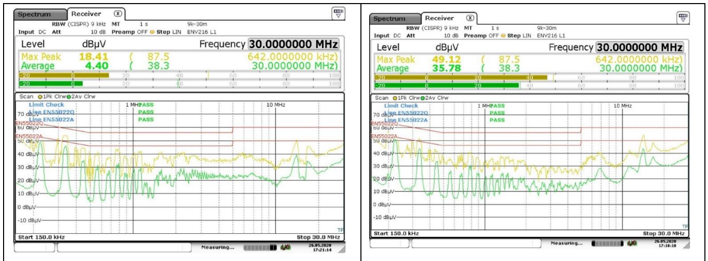
Figure 27 Conducted emissions at 230 V AC and 20 V/3.25 A load; neutral (left), live (right)
