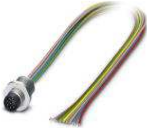
Sensor/actuator flush-type plug, 8-pos., M8, front/screw mounting with M10 fastening thread, with 0.5 m TPE litz wire, 8 x 0.14 mm 2
