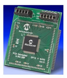
Processor Plug-In Modules are small circuit boards to be used with the various Microchip Development Boards to evaluate various MCU families. These plug into the main processor socket of the Development Boards so that different microcontrollers can be used for prototyping, demonstration or development --quickly and easily.
