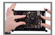
Similarly, it is recommended to plug back in the Processor Module by pressing down on the sides of the Processor Module as shown in the picture to minimize risk of
