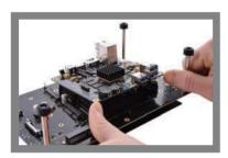
If necessary to unplug the Processor Module, it is recommended to do so by pushing up from the corners as shown in the picture to minimize risk of
