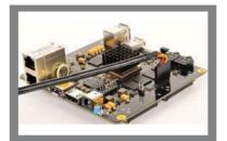
Connect the supplied USB to serial cable to the processor board as shown (for simplicity only the processor board is shown).
