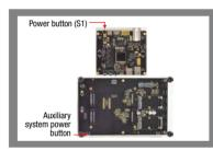
To turn on, press and release power button (S1) or auxiliary power button. To turn off, press and hold the same button for 15 sec. Do not unplug the power supply to turn off the board, as it may cause damage.
