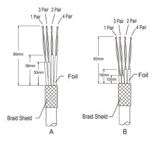
3. Refer to color coding on labels, allocate the pairs according to color coding in sequence, use punch down tool to press each conductor and trim excess length until all pairs are terminated.
