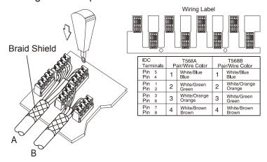
Place grounding clip on the cables, screw on the bolt until the cables are fastened to secure grounding between cable and panel.
