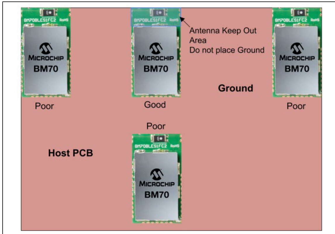
FIGURE 4-3: BM70BLES1FC2 ANTENNA PLACEMENT EXAMPLES
