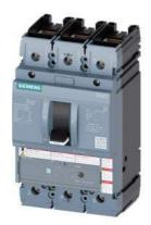
circuit breaker 3VA5 UL frame 250 breaking capacity class C 100kA @ 480 V 3-pole, line protection TM240, ATAM, ln=100A overload protection lr=80A ...100A short-circuit protection li=5...10 x ln cable connection on both sides
