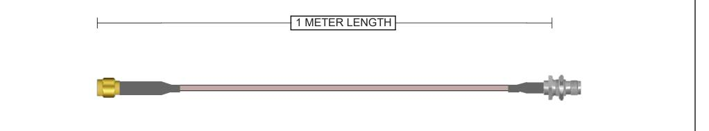
Connector A 132114RP SMA Plug Straight Brass Gold + Heatshrink 50 Ohm RG-316 Continuity/Hi-Pot Connector B 122428 TNC Jack Straight Bulkhead - Rear Mount Brass Nickel + Heatshrink
