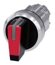
Selector switch, illuminable, 22 mm, round, metal, shiny, red, selector switch, short, 3 switch positions I>O<II, momentary contact on the left, latching on the right, actuating angle  $2x45^{\circ}$ , 10:30h/12h/13:30h
