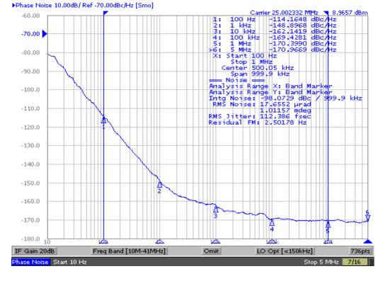
2.5V Core/2.5V Output **RMS phase jitter (Random)** 100Hz to 1MHz =0.112ps (typical)
