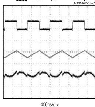
MEDIUM-LOAD SWITCHING WAVEFORMS (V IN = 3.8V, V OUT = 1.8V, I LOAD = 300mA, SKIP = BATT)
