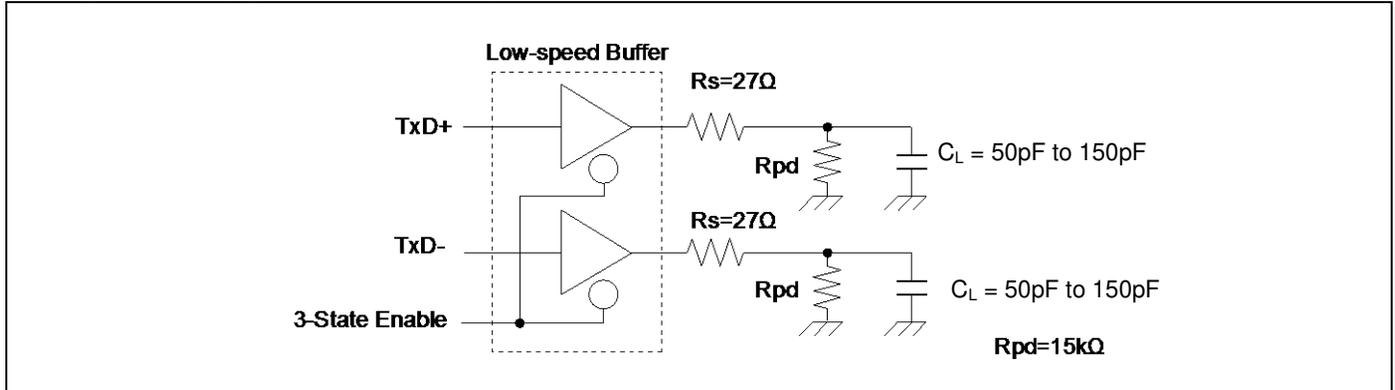
**Low-Speed Load (Downstream Port Load) - Reference 2**
