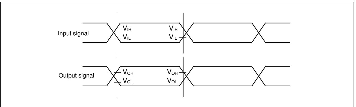
**Separate Bus Access Asynchronous SRAM Mode**
