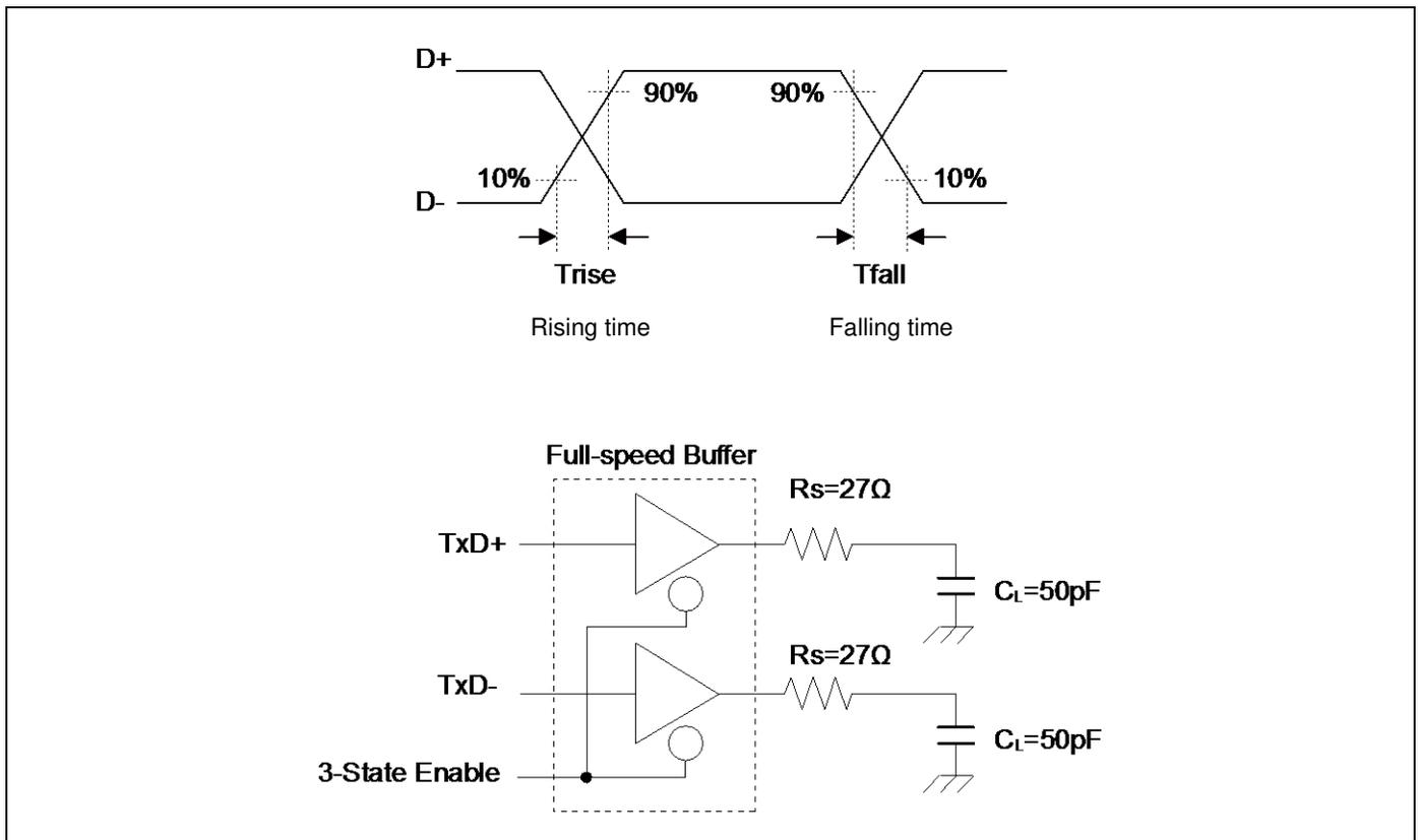
\*6: USB Full-speed connection is performed via twist pair cable shield with  $90 \Omega \pm 15\%$  characteristic impedance (Differential Mode).
