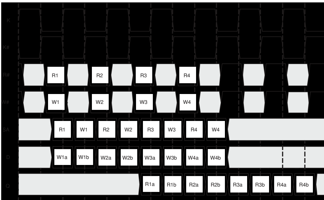
Figure 75. ORSPI4 Memory Controller Interface to QDRII: 2-Word Burst Mode
