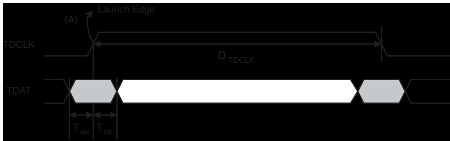
Figure 91. SPI4.2 Transmit Timing Points with Respect to Clock Edge
