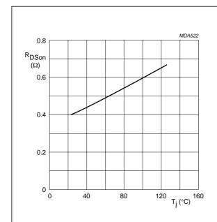
$I_D = 2.4 \text{ A}; V_{GS} = 10 \text{ V}.$
