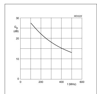
Class-B operation;  $\rm V_{DS}$  = 28 V;  $\rm I_{DQ}$  = 2  $\times$  80 mA;  $\rm P_{L}$  = 80 W.
