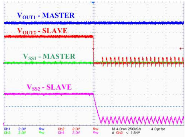
Figure 62. Master Voltage – End of Augmented OLM
