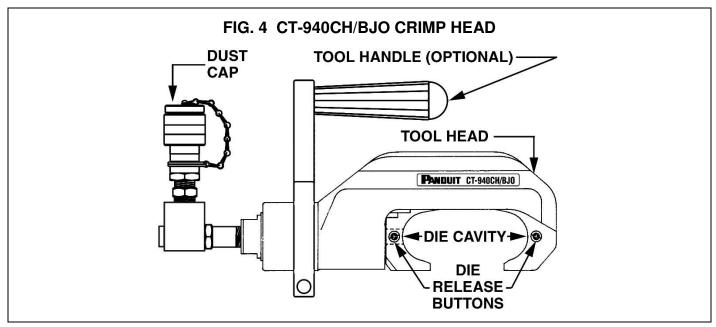
NOTE: The optional tool handle (CT-940CHHAN) is recommended for ease in carrying when the crimp head is being moved frequently.
