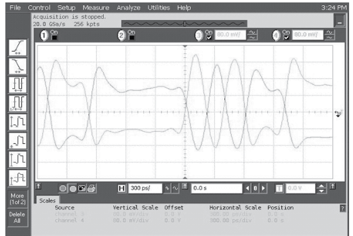
Data Waveforms, 3.0Gbps (left) & 6.0Gbps (right)
