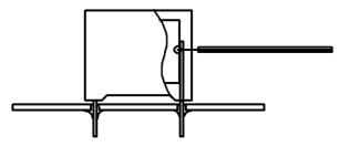
Temperature monitored inside the capacitor.
