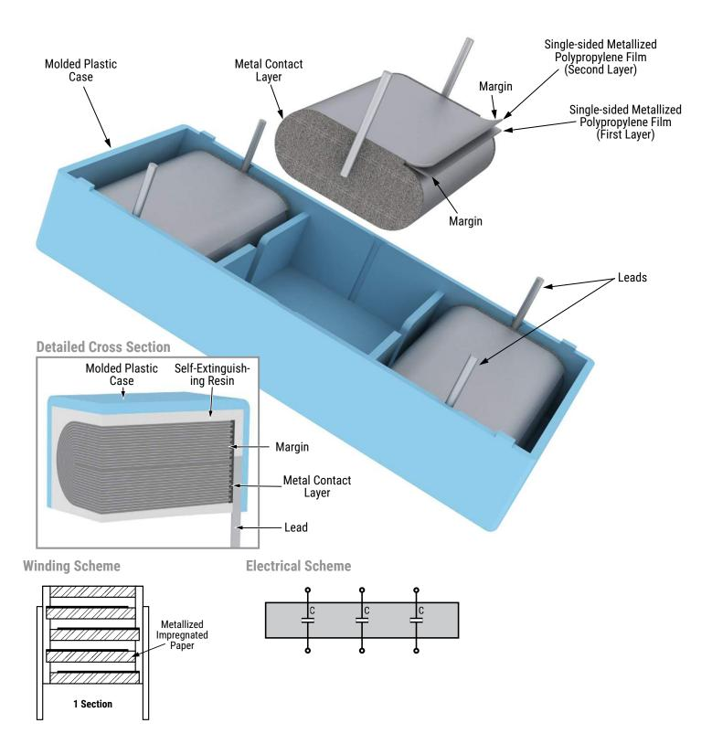
**OBSOLETE** Film Capacitors – AC Line EMI Suppression and RC Networks PHZ9004 Series Metallized Polypropylene Film, 300 VAC 3x X2 with Separate Terminals for Three-Phase Filtering
