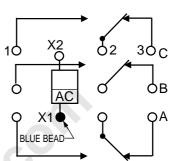
**NOTE:** Polarity must be observed with DC coil supply. Relay is polarized with a permanent magnet and will not operate or be damaged by reverse polarity.
