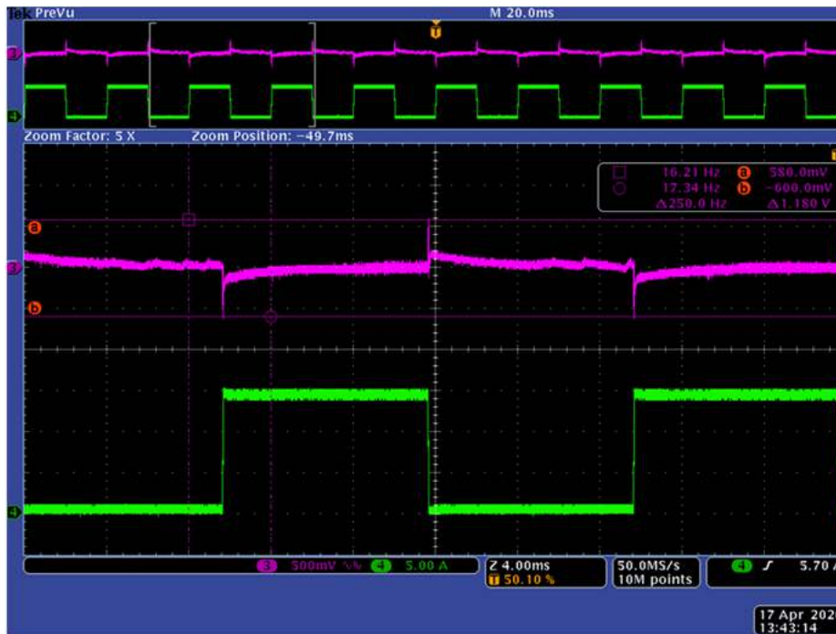
Figure 19. No Load to Full Load Transient Zoomed In (CH3=LLC Output AC Coupled; CH4=Output Current)
