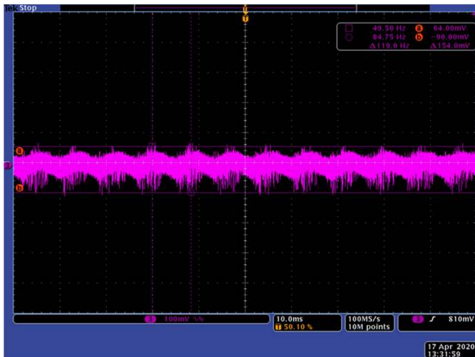
Figure 17. Full Load Output Ripple (CH3=LLC Output AC Coupled)
