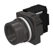
30mm BlackMax, Epoxy Coated Corrosion Resistant Complete Metal Unit Illuminated Push-Pull Operator Full Voltage, 6V AC/DC Incandescent Lamp Less Mushroom Head Cap 3 Position Pull-Momentary/Push-Maintained UL Listed, CSA Certified NEMA 1,3,3R,4,4X,12,13 & Automotive Standards
