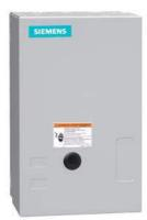
Non-reversing NEMA contactor, Size 2, Three phase full voltage, Contactor amp rating 45A, 3 wire (NO aux included), 190-220/220-240V 50/60Hz coil, Non-combination type, Enclosure NEMA type 1, Indoor general purpose use, Standard width enclosure
