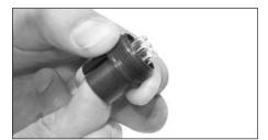
Step 3: Confirm insulator is fixed inside shell by applying slight force on the engaging side of the insulator. If properly installed, the insulator can not be pushed out the rear of the shell. If the insulator is displaced with this test, please repeat steps 1 and 2.
