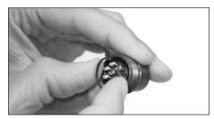
Step 2: After insulator is seated in shell, install the snap ring on the rear of the connector. Slightly compress ring and insert into recessed area just above the insulator. If not completely in place, manipulate the snap ring with finger until visual or audible seating confirmation is made. No tooling is required.
