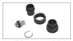
Unassembled connectors are supplied in kits, an insulator kit and hardware kit. The insulator kit includes a snap ring and insulator with preloaded contacts. The hardware kit includes the shell along with appropriate endbell (except box mount receptacles) and coupling nut (plug only).
