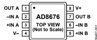
Figure 2. 8-Lead MSOP (RM-8)
