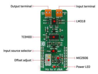
When Hz to V click is operated for the first time, it needs to be calibrated. The click is equipped with a variable resistor for the offset fine tuning. The following procedure should be followed to calibrate the device:
